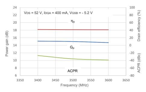
Fig 3. Single-Carrier WCDMA broadband performance @ Pout = 48.5 dBm Avg.
