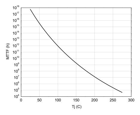
Fig 5. Median lifetime vs. channel temperature
