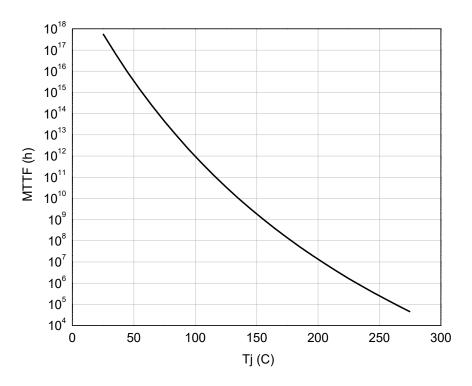
Fig 5. Median lifetime vs. channel temperature
