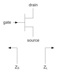
Fig 3. Definition of transistor impedance
