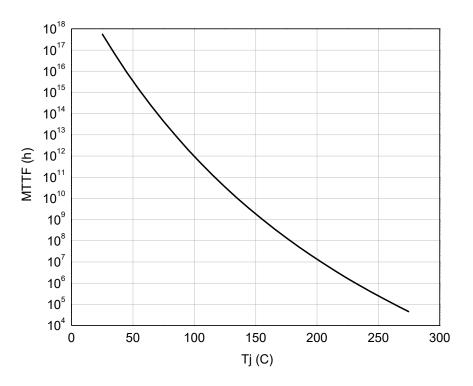
Fig 4. Median lifetime vs. channel temperature
