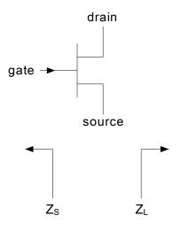
Fig 5. Definition of transistor impedance
