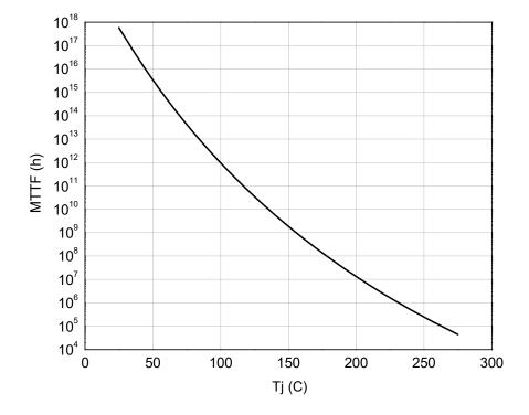
Fig 6. Median lifetime vs. channel temperature
