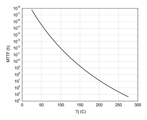
Fig 5. Median lifetime vs. channel temperature
