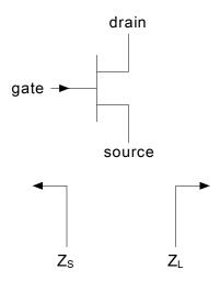
Fig 4. Definition of transistor impedance
