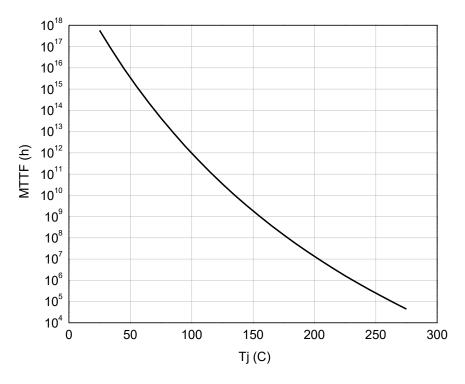
Fig 5. Median lifetime vs. channel temperature
