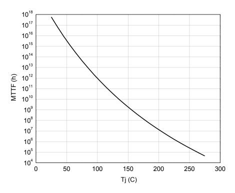
Fig 5. Median lifetime vs. channel temperature
