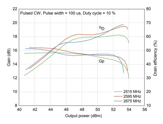
Fig 3. Power gain, Drain efficiency vs. Pulse output power
