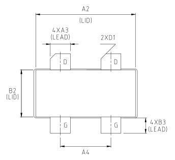
PINS: D--drain G--gate S--source
