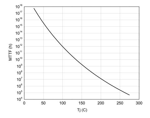
Fig 4. Median lifetime vs. channel temperature
