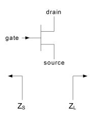
Fig 3. Definition of transistor impedance
