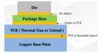
Figure5. Thermal Model Stack-up for DFN Package.
