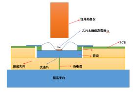
Figure2. The test diagram of IR.
